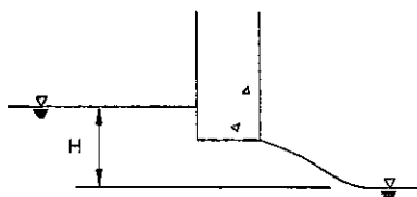
When Riser Box Elev. > Center of Orifice
